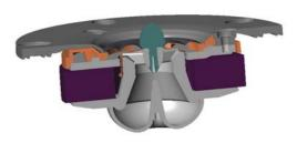
resulting in zero, or very limited output from the tweeter. By clamping the middle of the dome and only using a ring of the cone area on each side of the voice coil, the tweeter is able to reproduce frequencies up to 40kHz.
